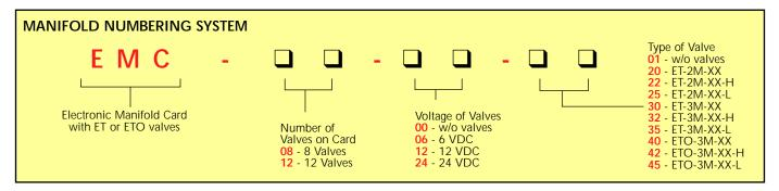
EMC-08-00-01 and EMC-12-00-01 are part numbers for cards without any valves, and without manifold. Manifold mounting hardware is included. Manifolds may be ordered separately, if desired.
